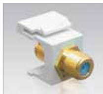
F-type Video IC107B9Gxx* F-type female to female, gold, 3 GHz
